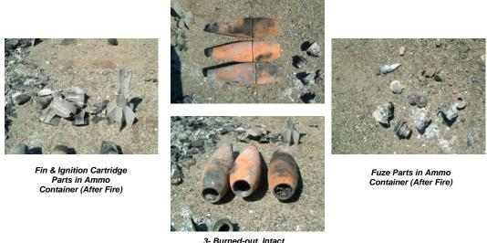
3- Burned-out, Intact Projectile Bodies in Ammo Container (After Fire)
