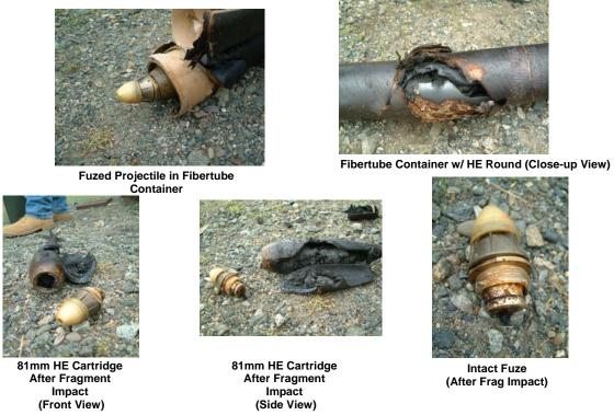
Figure 2: Fragment Impact Results for 81mm Mortar, Test #2 – Type V Reaction
